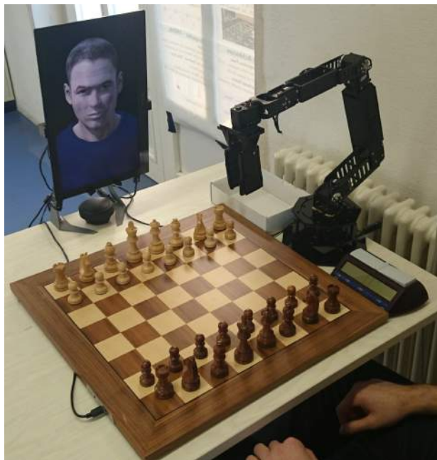
Figure 1. The pan-tilt-roll agent display, the robotic arm, and the digital chess board together with the digital chess clock
