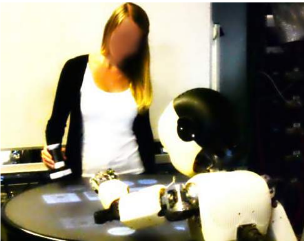
Figure 2. Experimental setup of the robot interacting with a human using the Reactable for the educational game scenario. In the image you can see the participant holding an object used to select an item from the Reactable (round table with projected images of countries and capitals). The participant is facing the iCub. The projected items are mirrored, so each side has the same objects.
